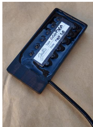
Figure 2 - The back of the pickup, showing the cable. It extends around 15 cm.
