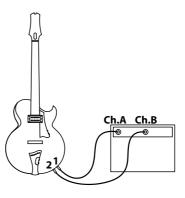
You must remove the cable from #2 when you are done playing; otherwise the battery will deplete.
