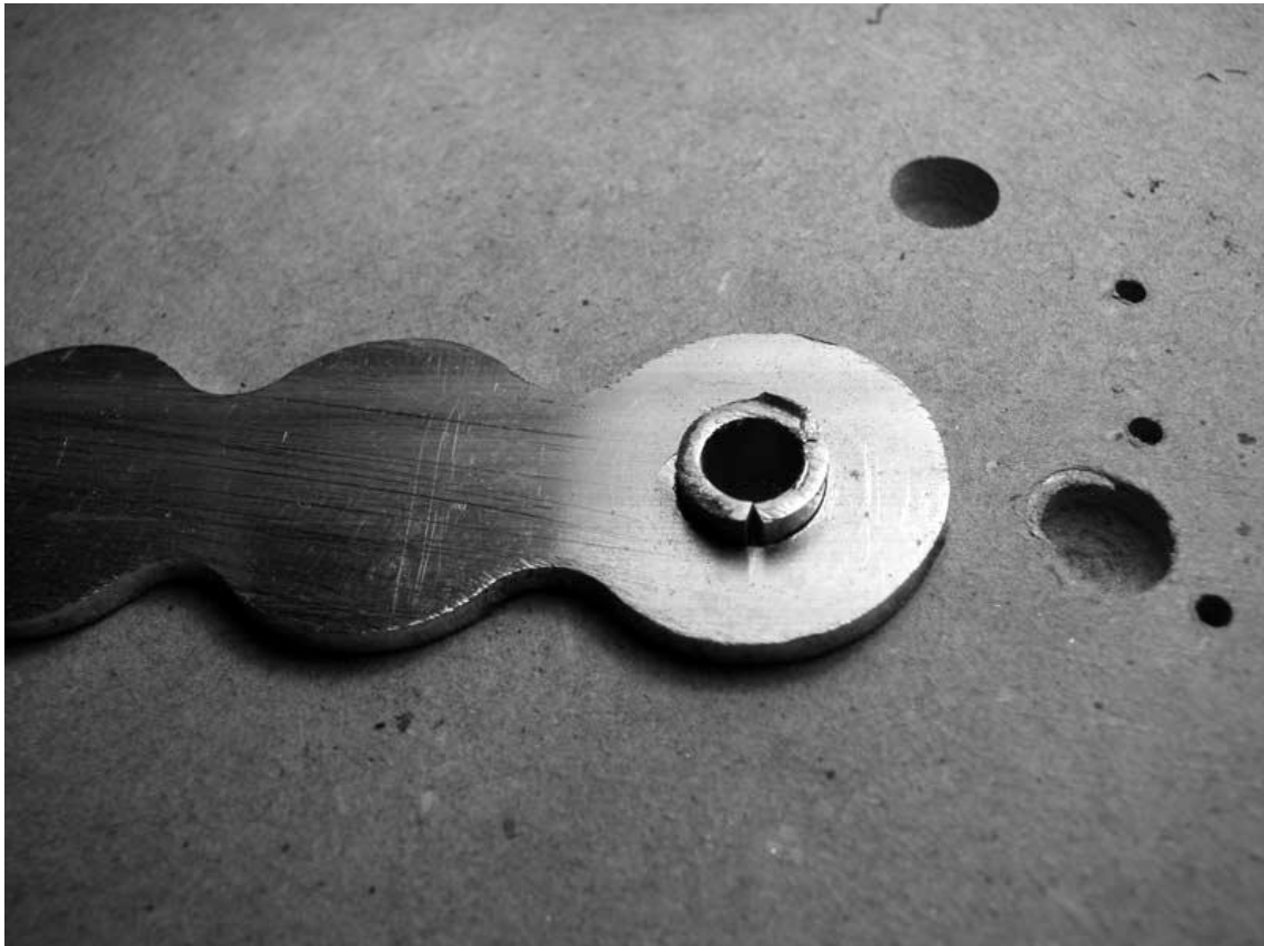
This is the bracket after sanding the overhang:
